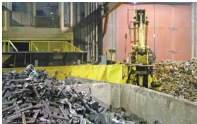
Fig. 5. Cut off sprues, runners and gates are saved as foundry returns to be remelted for more castings.
