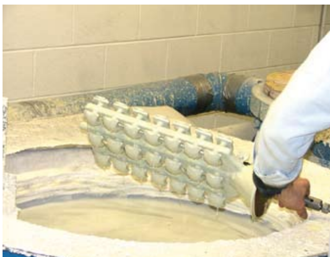
Fig. 9. In investment casting, wax patterns are dipped into a mixture of refractory materials, called a slurry, which is then fired and dried before molten metal is poured into the mold.
