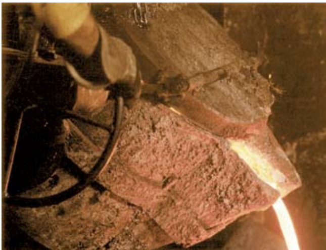
Fig. 7. Molten metal is poured from a ladle into a mold.
