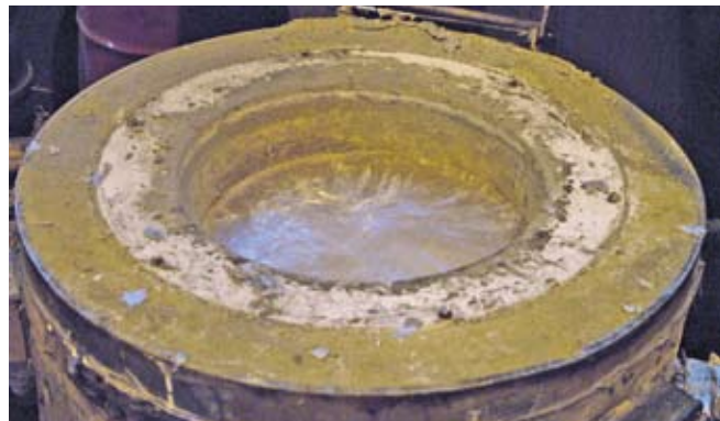
Fig. 1. Molten metal in a furnace, crucible or ladle is referred to as the bath.
