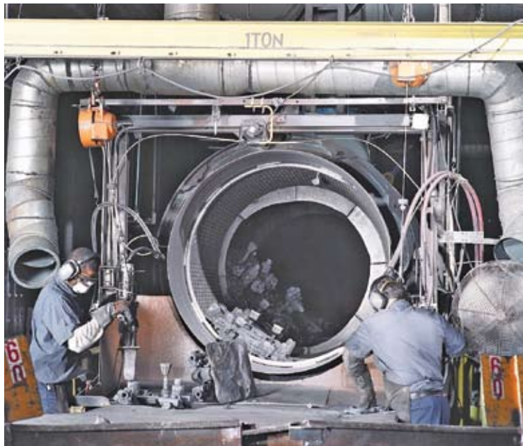
Fig. 8. In this form of shakeout, castings are tumbled out of their sand molds while workers wait at the end to detach the gates, runners and sprues with pneumatic wedges.
