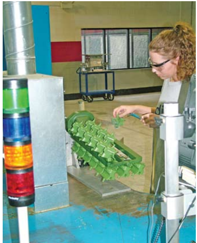
Fig. 10. Wax patterns are affixed to an investment tree. These patterns will eventually be coated in a slurry and burned out to leave hollow cavities.
