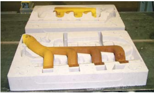
Fig. 3. Cores are placed into a mold.
